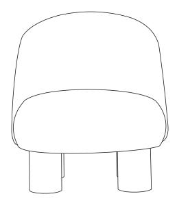
Legs and Hardware are located inside the product. Attach 4 x legs (2) to 1 x base (1) as shown and turn to tighten.
